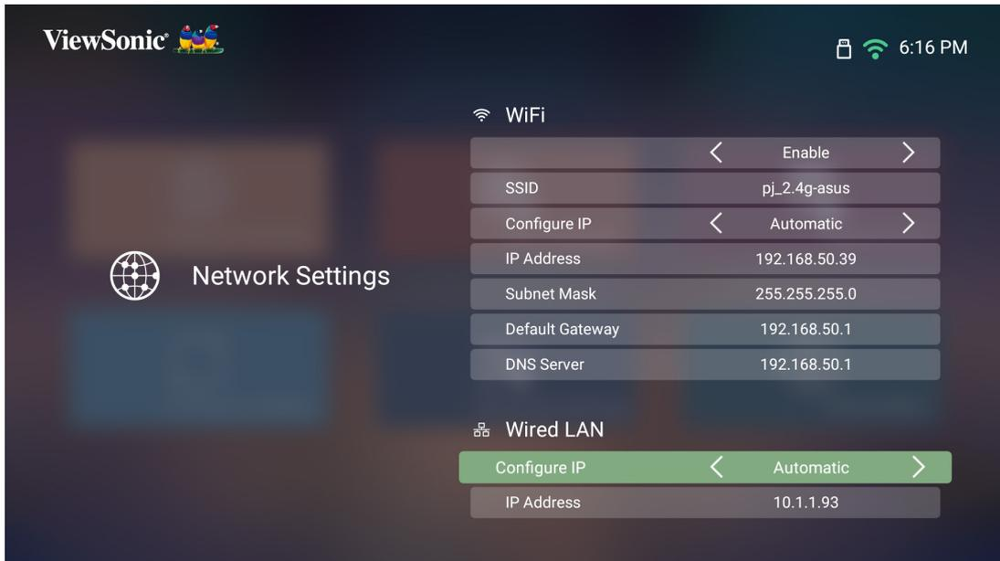
3. You can Configure the IP automatically or manually. Choosing **Manual** will allow access to **IP Address, Subnet Mask, Default Gateway, and DNS Server.**
