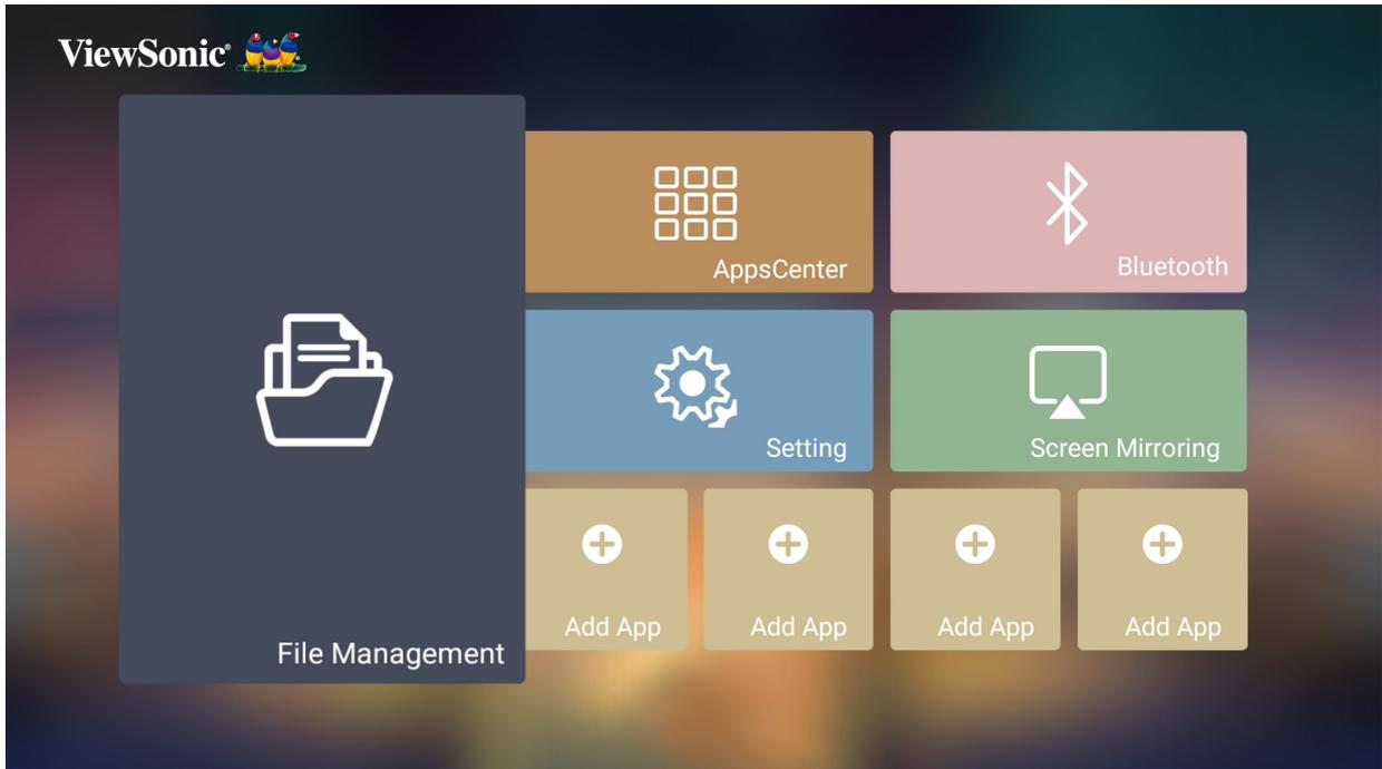
2. Select a device on the source list: USB, Local Storage, etc. Use the direction buttons to select the desired file. Then press **OK** on the remote control to open the selected file.
