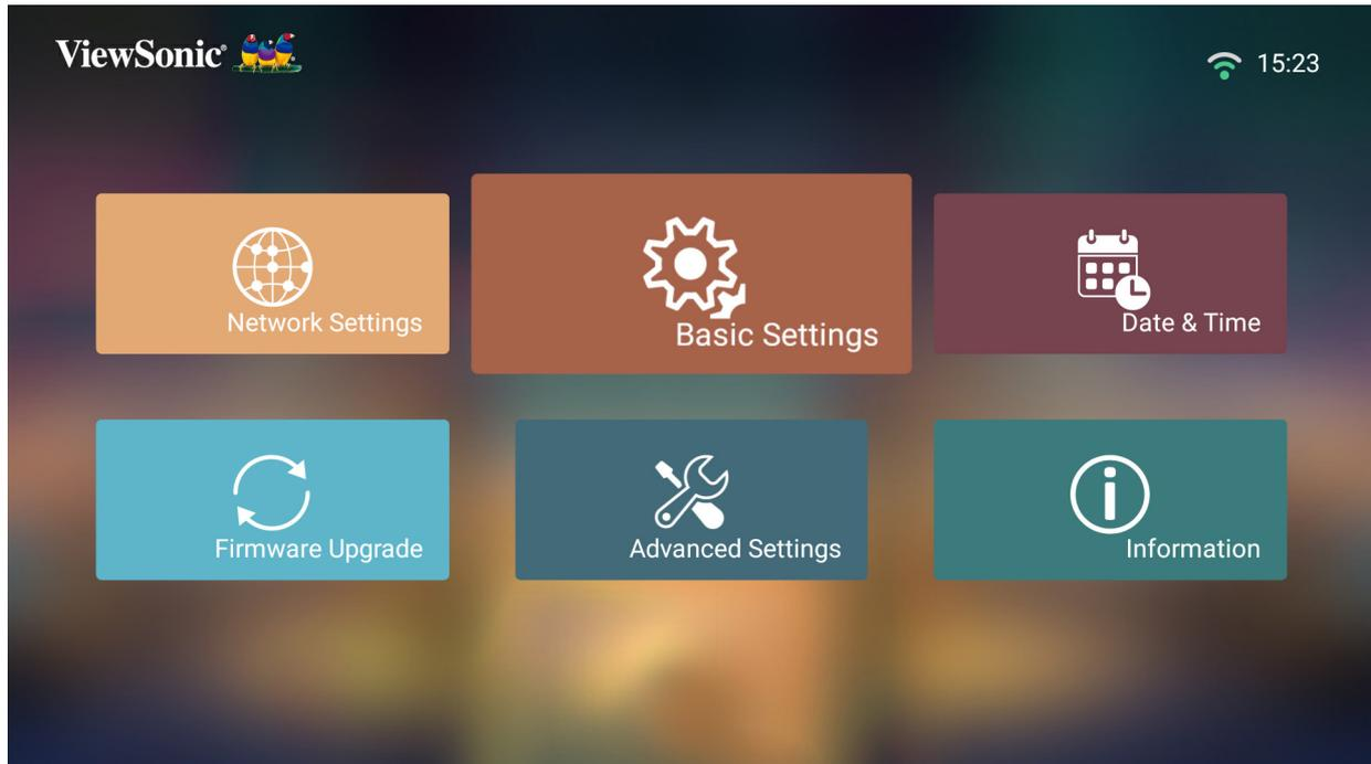
2. Use the **Up** and **Down** buttons to select the desired option and press **OK**. Then use the **Left** and **Right** buttons to make adjustments or selections.
