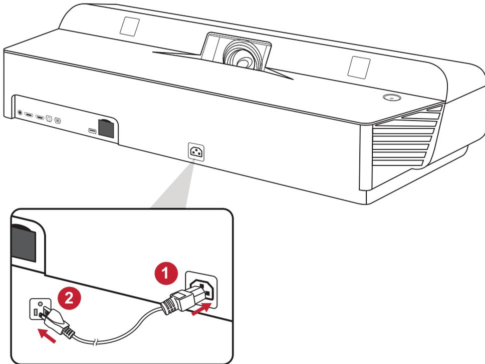
**NOTE:** When installing the projector, incorporate a readily accessible disconnect device in the fixed wiring, or connect the power plug to an easily accessible outlet near the unit. If a fault should occur during operation of the projector, use the disconnect device to switch off the power supply, or disconnect the power plug.
