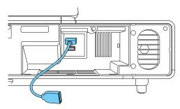
Connect the USB power cable supplied to the DC Out (2.0A) power supply port.
