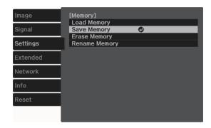
Use the up and down buttons to select the memory name you want to save, and then press the [Enter] button to confirm the selection.
