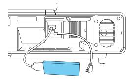
Connect the USB power cable to the USB port (type B) on the streaming media player.
