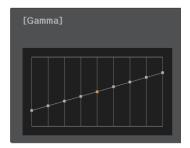
Use the up and down buttons to adjust the brightness, and then press the [Enter] button to confirm the selection.
