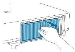
Hold the air filter with the surface facing down and tap it 4 or 5 times to remove the dust.
