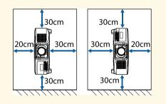
• Do not install the projector in a location that does not allow air to circulate, such as on a shelf or in a box.
