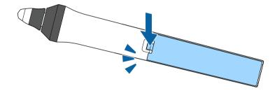
Two interactive pens come with two types of pen tips, soft tips and hard tips. The soft pen tips are installed on the pens by default.
