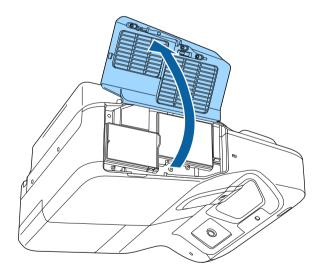
Pull the air filter out of the projector.
