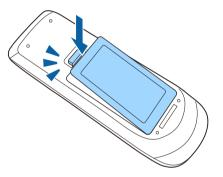
The Interactive pen uses one AA manganese battery, AA alkaline battery, or Eneloop (BK-3MCC) rechargeable battery. Replace the battery as soon as it runs out.
