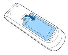
Insert the batteries with the + and - ends facing as shown.
