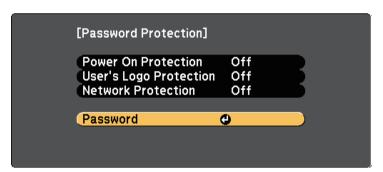
If you do not see this menu, hold down the [Freeze] button on the remote control for 5 seconds until the menu appears.
