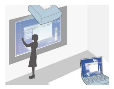
When the projector is connected to a computer with a USB cable, you can operate the computer from the projected screen using the interactive pens or your finger (EB-695Wi/EB-680Wi), just as you would with a mouse. You can navigate, select, and interact with your computer programs from the projected screen.
