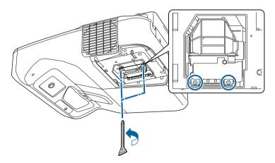
Grip the lamp handle and carefully pull the lamp out of the projector.
