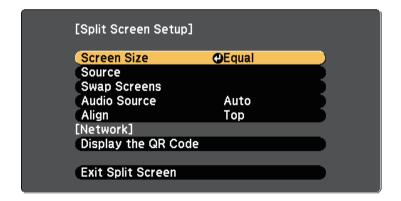
To select an input source for the other image, select the **Source** setting, press [Enter], select the input source, select **Execute**, and press [Enter].
