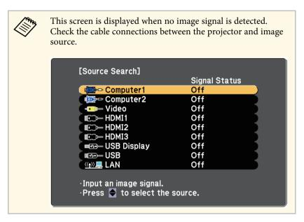
• Press the button for the source you want on the remote control. If there is more than one port for that source, press the button again to cycle through the sources.
