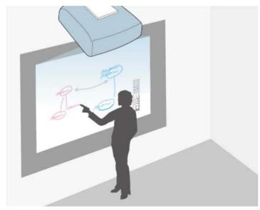
You can use the interactive pens or your finger (EB-695Wi/EB-680Wi) to write or draw on the projection surface just as you would on a chalkboard or dry erase board.
