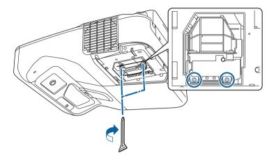
**9** Replace the lamp cover and tighten the screw to secure it.
