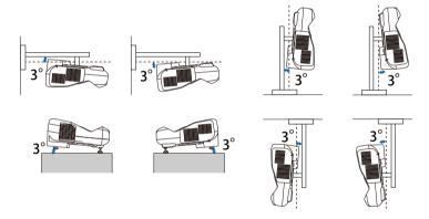
If you use the projector tilted at an angle of more than 3° it could be damaged and cause an accident.
