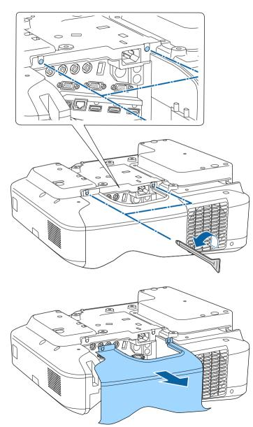
Connect the Wireless LAN module to the wireless LAN module slot.
