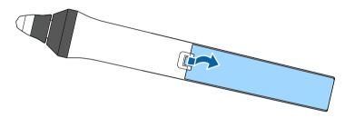
Insert the battery with the + and – ends facing as shown.
