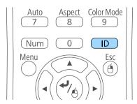
The current Projector ID is displayed on the projected screen. It disappears after about 3 seconds.
