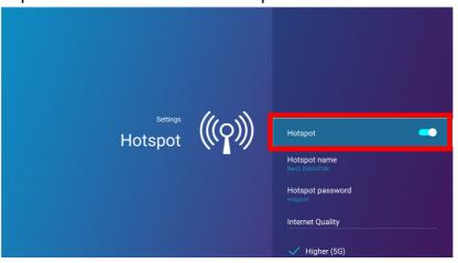
8. Once wireless hotspot is enabled, use the name shown in the **Hotspot Name** field as the SSID to connect to from your mobile device's wireless menu and use the password shown in the Hotspot Password field as the connection password.
