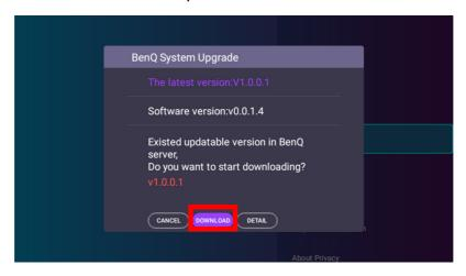
2. Once the download is completed, the projector will restart automatically. Do not turn off or unplug the projector before the projector is finished updating and **BenQ Launcher** reappears on the screen.
