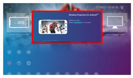
2. On your Android mobile device's wireless network menu connect to the wireless network shown on the Wireless Projection for Android™ screen and then select Next.
