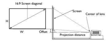
• The screen aspect ratio is 16:9 and the projected picture is in a 16:9 aspect ratio
