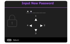
5. To activate the **Power On Lock** function, press  $\triangle/\nabla$  to highlight **Power On Lock** and press **◄/▶** to select **On**. Input the password again.
