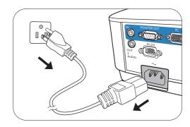
3. Once the cooling process finishes, the power indicator becomes a steady orange and fans stop. Disconnect the power cord from the power outlet.
