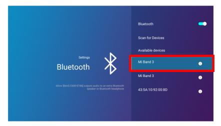
8. When the projector and speaker or headphones have successfully connected the device listing in the Bluetooth setting menu will be labeled **Connected**, you can now output the audio from the projector to the speaker or headphone.
