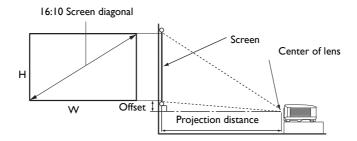
• The screen aspect ratio is 16:10 and the projected picture is in a 16:10 aspect ratio
