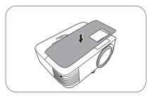
13. Tighten the screw that secures the lamp cover.
