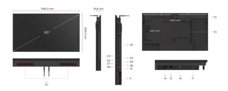
1. Speaker 2. OPS Slot 3. USB 2.0 4. RS-232 5. USB 3.0 6. USB-C 7. HDMI 1(ARC) 8. HDMI 2 9. HDMI OUT 10. HDMI 3 11. Control Panel 12. WiFi Slot 13. VESA® Wall Mount (600x400mm) 14. AC IN
