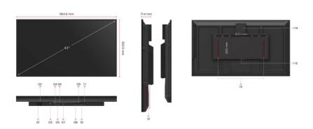
1. Power Switch 2. AC IN 3. SPDIF 4. LAN 5. USB 2.0 6. USB 3.0 7. RS-232 8. HDMI OUT 9. HDMI 2 10. HDMI 1(ARC) 11. USB-C 12. Control Panel 13. Speaker 14. WiFi Slot
