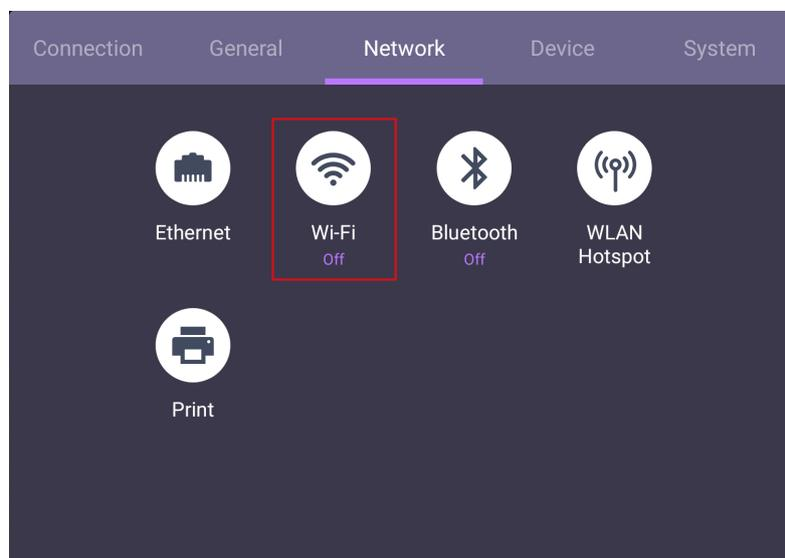
2. Insert the Wi-Fi dongle and the switcher will automatically change to **ON**. A list of available networks will show on the screen.
