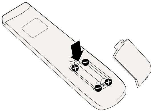
2. Insert the supplied batteries, ensuring that the positive and negative ends are facing in the correct direction.
